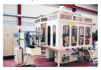
The conventional machining units, which are equipped with hydropneumatic or hydraulic feeds, offer a cheap and economical manufacturing concept, especially for simple parts, which can produce successfully for decades.
